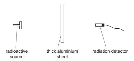
The radiation detector shows a reading greater than the background reading.
