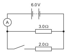
The switch is open, and the ammeter reads 2.0 A.
